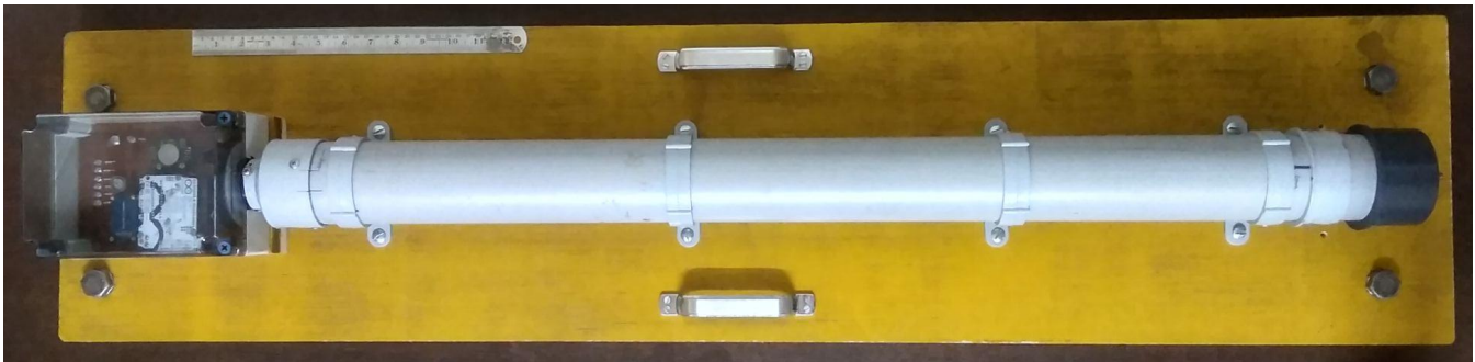
Figure 1a: The optical mouse-based seismometer. The pipe holds the cantilever and the box contains the circuit. The device is mounted on a wooden platform with adjustable height.
